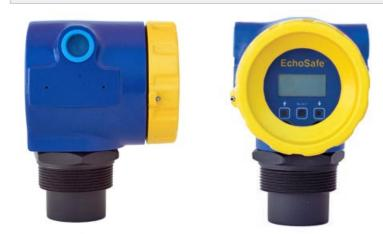
FM approved for hazardous environments, the explosion proof ultrasonic level transmitter provides continuous level measurement up to 32.8' (10m) with a 4-20 mA signal output, and is configured via the integral push button display module. This non-contact liquid level sensor is ideally suited for corrosive, ultrapure, sticky or dirty liquids, and is widely selected for bulk storage, day tank, lift station and process tank level applications located in a classified area.
