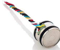
SERIES PD 9 L DIFFERENTIAL Ø 19 x 14 mm, wet/wet 0,1...50 bar diff. Line pressure max. 200 bar
