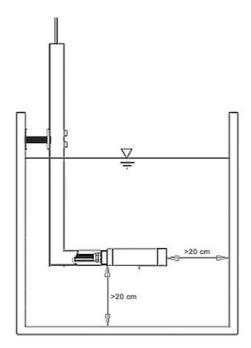
Install the probe in the channel so that it is immersed for at least 20 cm and the distance from walls and bottom of the channel is not less than 20 cm.
