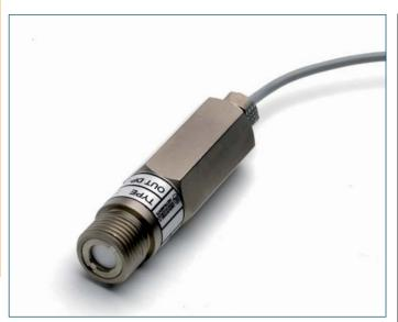
The SF52 dew-point transmitter from Michell Instruments can provide 4–20 mA or voltage signal for either dew point or absolute humidity with excellent accuracy and linearity. The robust housing, together with an operating pressure of up to 20 bar (290 psi), makes the SF52 ideal for many dew-point and moisture measurement applications.
