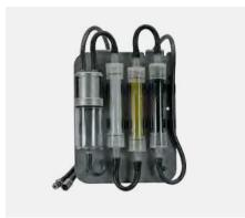
Mini filtering plate with multistep gas process (plate hooked at analyser): Gas drying in the water trap-Prefiltering thru fine dust filter – Additional drying thru silicate gel – Sensor-toxic, organic compounds captured by the hydrocarbon filter.
