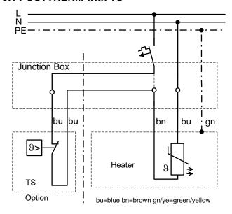
Connection cable Silflex-EWKF 3x1,5 mm<sup>2</sup>, 1m long. Other lengths available upon request (at an extra charge).
