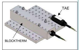
The block heater dissipates the heat by conduction. It should be mounted to a flat surface of a heat conducting material (e.g. metal). 2 bolts are sufficient to mount the heater.
