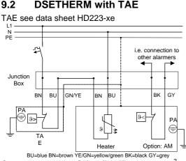
Connection cable Silflex-EWKF 3x1,5 mm<sup>2</sup>, 1m long. Other lengths available upon request (at an extra charge).
