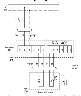
The above electrical wiring diagram is valid for a system up till 500 W with one heater. For more powerful systems with more than one heater an individually designed wiring diagram is supplied.
