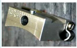
Picture 4 (The temperature sensor holder)
