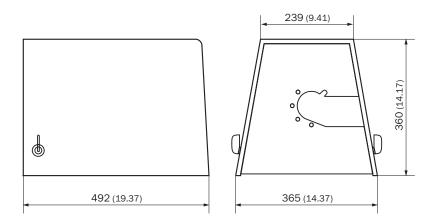
Weather hood for SLV4/SLV5/SLV7 purge air unit
